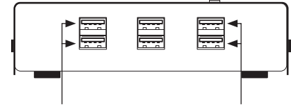
Up to 4 individual VB or VT series body-worn cameras can be connected to the ports shown.
